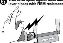
With lever open, tighten knob until the lever closes with FIRM resistance.
