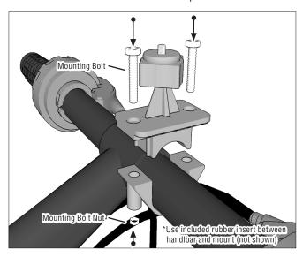
2 Attach Camera or other device with 1/4" 20 mounting pattern to mounting screw on the mount
