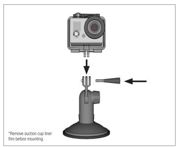
Clean surface with included alcohol pad. Firmly place mount on dash and engage suction lock lever.
