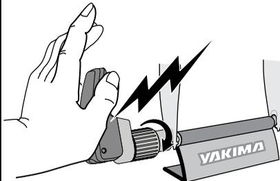
Loosen or tighten the knob as needed so that lever closes with **FIRM** resistance.
