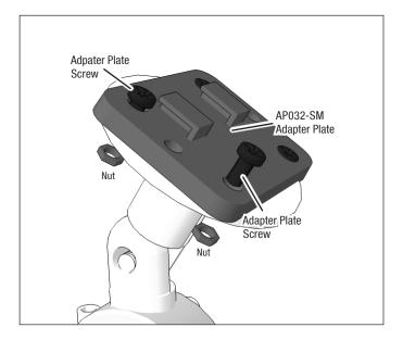
Separate mount clamp by unscrewing the Clamp Bolts with appropriate hex key and place mount on handlebar where desired; reassemble mount clamp using appropriate reducer bushings if necessary
