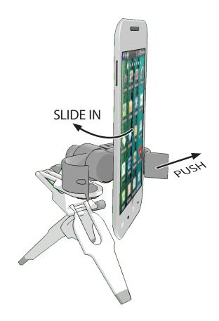
To remove, place your thumb on the holder arm and press gently until the phone releases outward.
