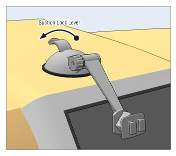
Attach any Arkon D ual-T Holder the the Dual-T Tabs on the Mount and adjust the heigh if the arm if necessary
