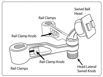
Adjust the lateral position of the swivel ball head and tighten the head lateral swivel knob for optimum viewing angle.
