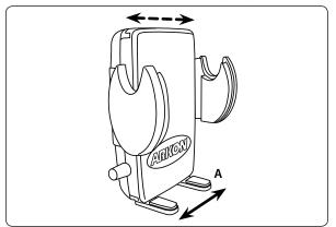
Step 2. Place device on the support legs (A) and squeeze the side grip arms (B) until they fit securely to the device.
