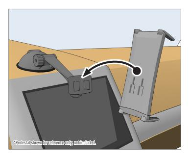
2 Push down lower legs of mount to insert device. Adjust position of holder as desired.
